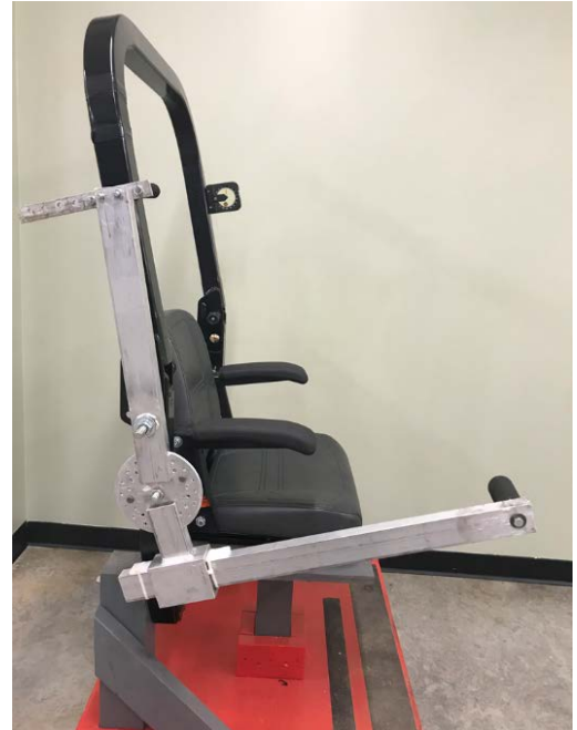
Universal lift assist lever mounted on a foldable ROPS.
